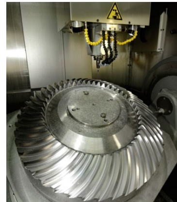
HERMLE C-50U ( m10, z47, \alpha20^\circ, \beta=35^\circ, d=470 )
