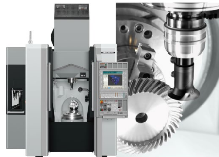
NMV3000 DCG ( m4, z40, \alpha20^\circ, \beta=35^\circ, d=160 )
