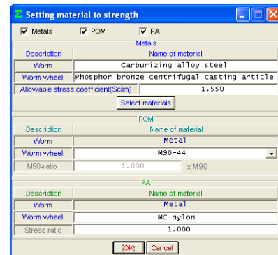
Fig. 3.13 Initial Strength Calculation Settings (with [Select Material] button)
