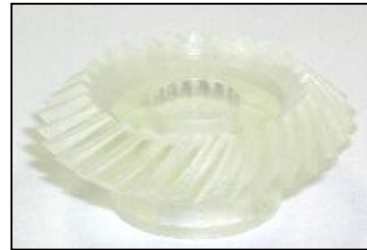
Fig. 2.38 Photo fabricated Gear Model (m1, NT28, \alpha 20°, \beta 35°)
