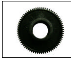
mn=0.5, Z=72, \alpha=20^\circ 射出成形歯車(POM)
