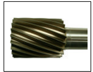
mn=1.39, Z=21, \alpha=20^\circ \alpha=20^\circ , 銅電極
