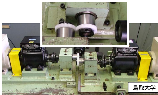
Fig.9 Photographs of test rig and test gears
