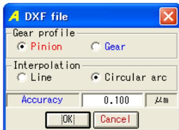
Fig 13. DXF file outputting form
